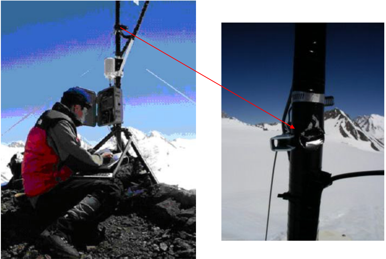
Fig. 5. AWS on the Fedchenko glacier. The right photo shows damage on the AWS mast caused by strong wind that broke down the solar panel and disrooted the electric supply cable.
